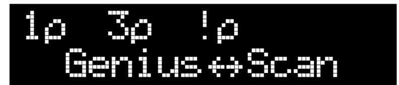
Figure 6e: Alternating "!" Indicates the Remote Needs to be Recharged
