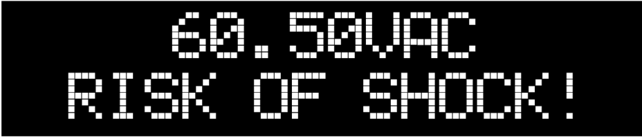
Figure 5c: Dangerous AC Detected
