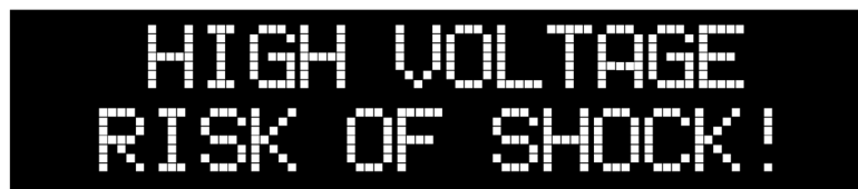
Figure 7f: Tone Mode Dangerous Voltage on F-Port
