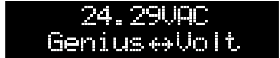
Figure 8b: 24.29 VAC Detected in Volt Mode
