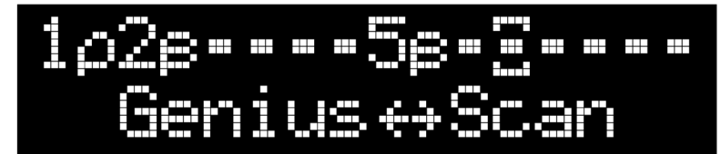
Figure 6a: Receiver Indicates Remote ID and Path Voltage Test Result
