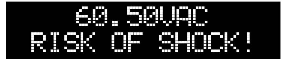
Figure 8c: Volt Mode Dangerous Voltage on F-Port
