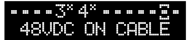
Figure 6b: Receiver Indicates Remote ID and Voltage on the Line
